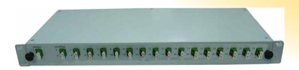
Splitter shelves are used for mounting MxN splitters. Rack mounted versions are designed for flange mounting on 19 inch racks. Fabricated from carbon steel, pre treated and painted with enamel or powder coated to ensure corrosion resistance. Standard mounting on 19 inch Finished in Standard colours of Siemens Gray or black, with other colours on request.
